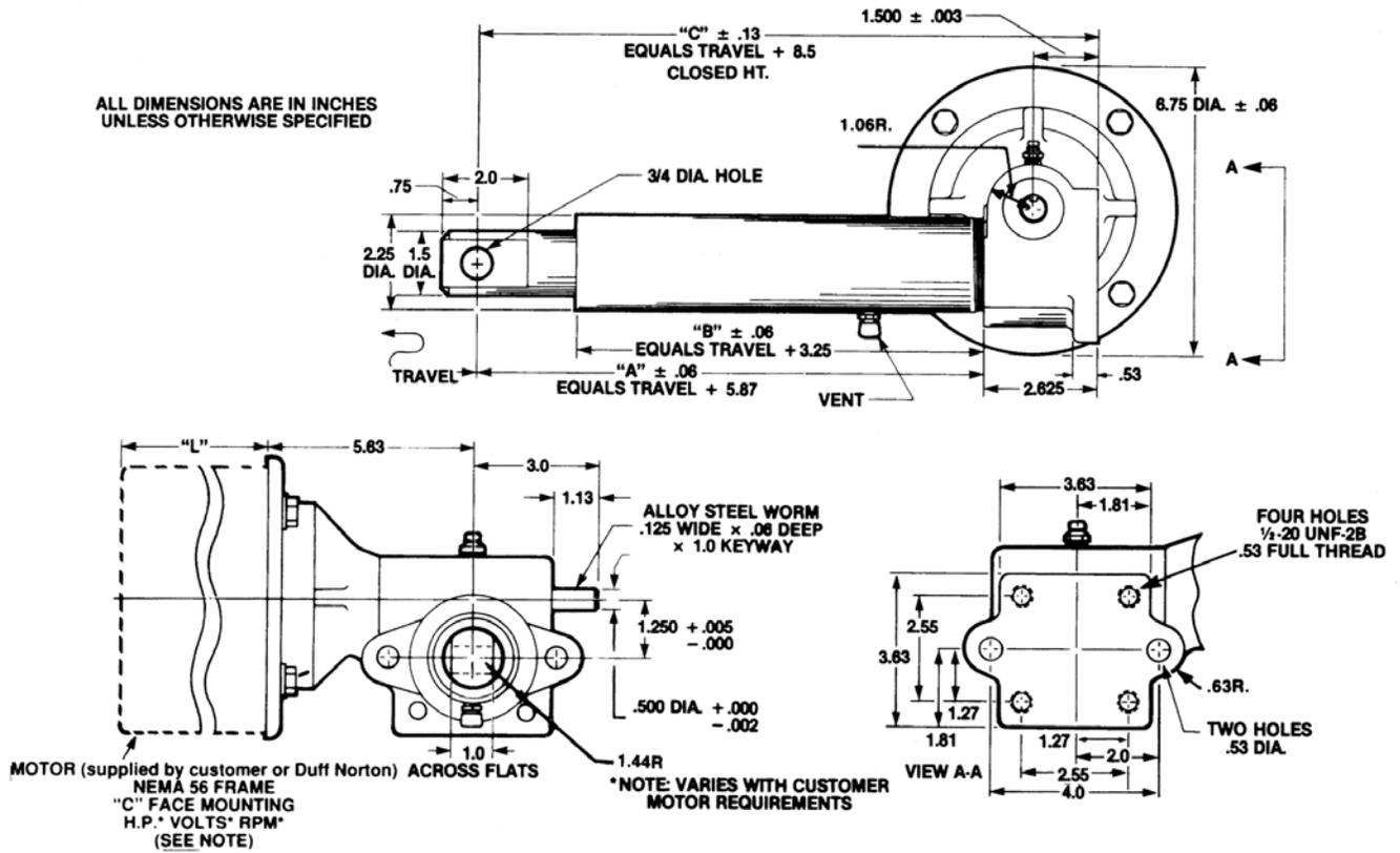
Figure 3-2. Dimensions - Translating Tube Actuators (Models M-2464 and M-2465)
