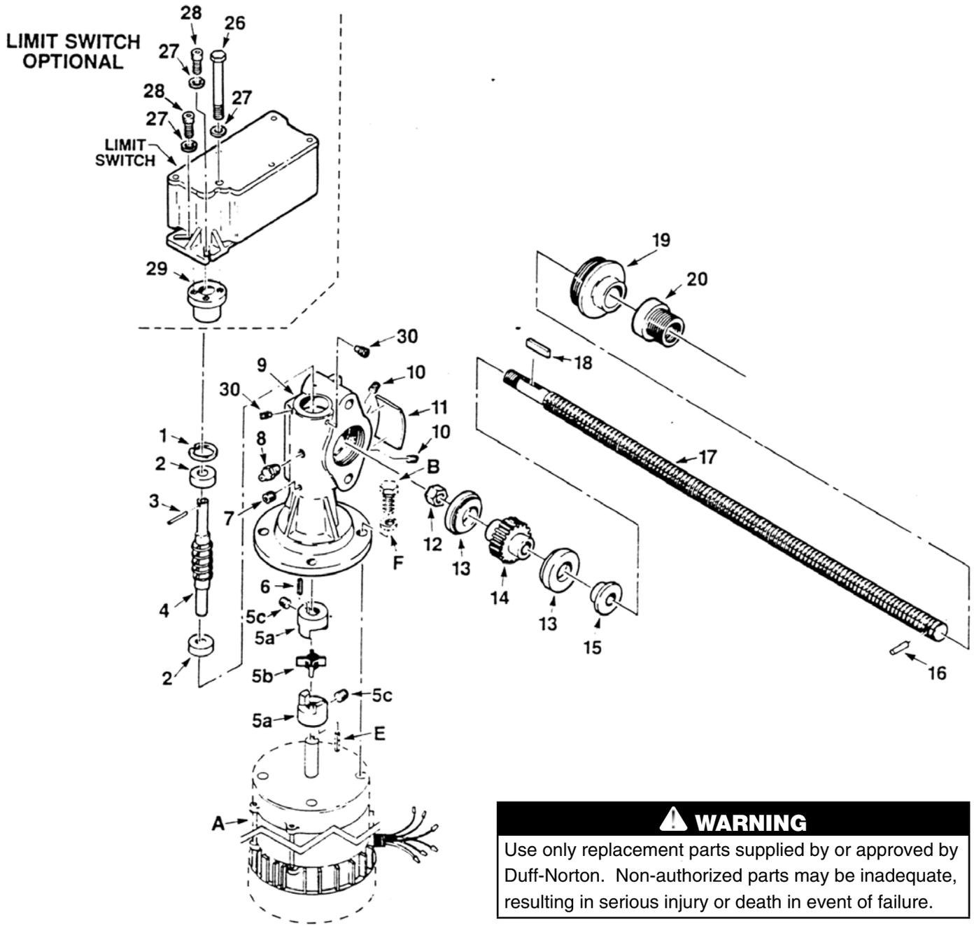
**Figure 6-1. Exploded Illustration Rotating Screw Modular Actuators (Models M-2464 and M-2465)**
