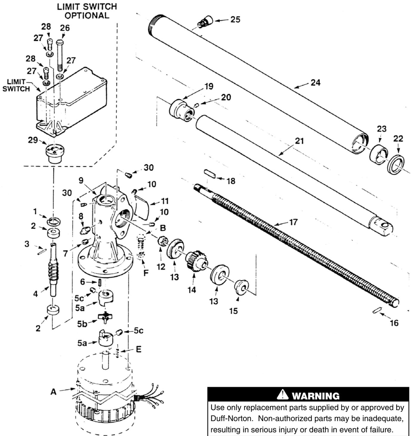
**Figure 6-2. Exploded Illustration Translating Tube Modular Actuators
