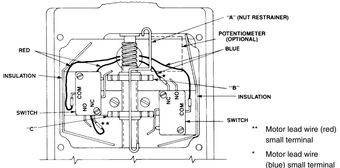
**Figure 6-3. Limit Switch Assembly, 6415 & 7415 Series AC Actuator**
