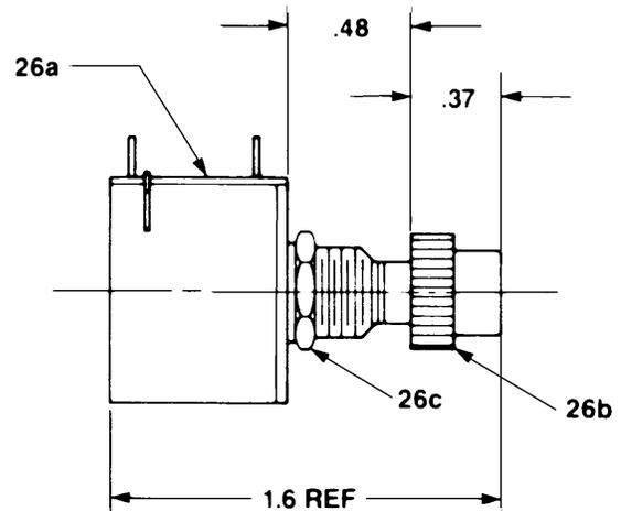
**Figure 4-1. Potentiometer Nut and Washer Assembly**
