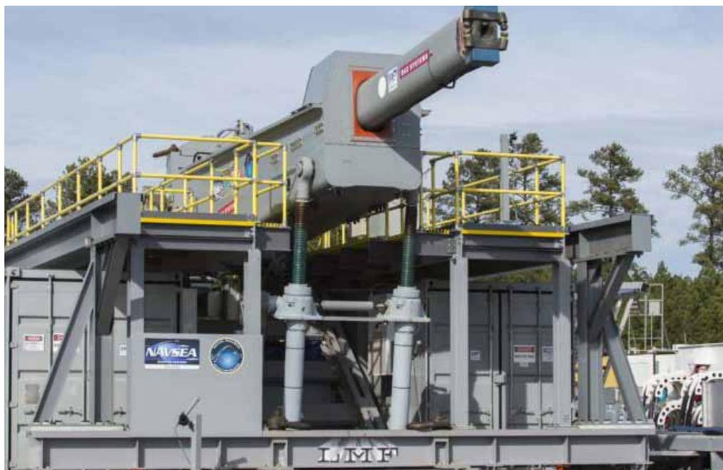
Shown front and center, a pair of Duff-Norton 150T Screw Jacks controlling the barrel elevation on the The Office of Naval Research (ONR) futuristic electromagnetic railgun. (Screenshot via Business Insider - Military & Defense)
