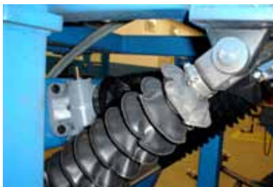
Translating actuator with bellow boot cover.
