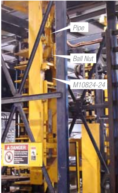
Automated concrete block lifting, stacking, and off-loading system.
