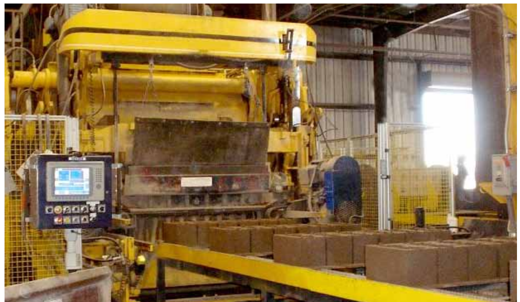
Concrete blocks on conveyer heading toward automated lifting, stacking and off-loading system.
