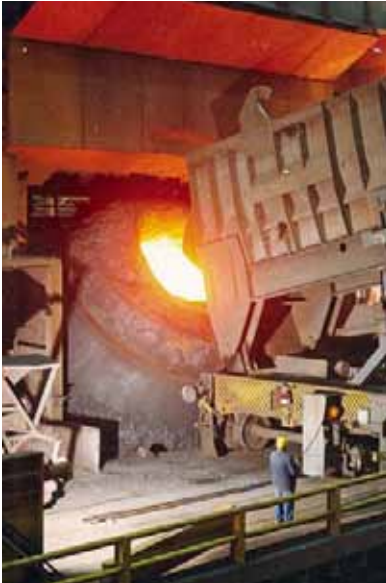
Alloy materials being poured into a BOF (shown for illustration purposes only)
