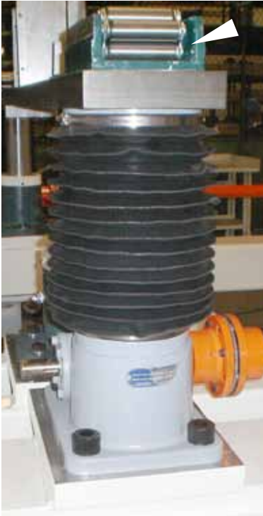
Close up of M1005-XXX screw jack which supports the base of the customer's carriage assembly.
