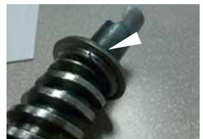
Distorted Flat Washer formed to the shape of the Acme Nut.
