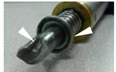
Direction of shear/fracture and deformed washer indicate compression force.
