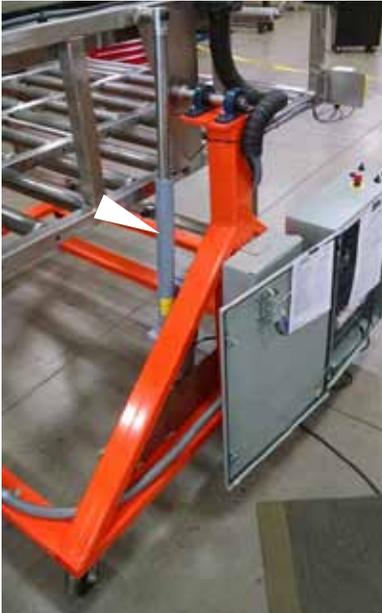
Fixture used to tilt evaporation coils showing SPA6415 Linear Actuator
