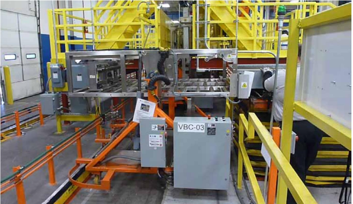
*Loading station. Coil is loaded from the right, then rotated to a vertical position.*
