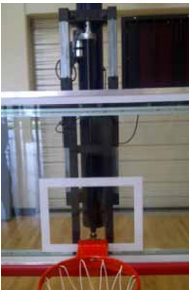
Front view of automated backboard with Duff-Norton Linear Actuator installed.
